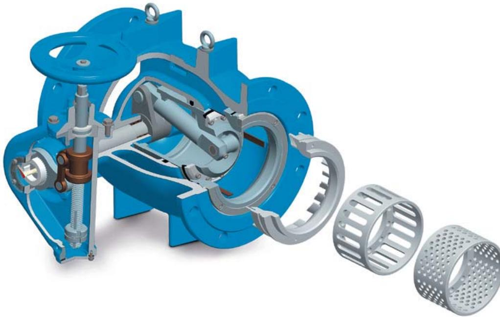
The valve body is double layer structure (inner and outer cylinder), crank mechanism converts rotation of the valve shaft to axial movement of the plunger along the guide rail which change the flow area between plunger and valve seat so that control the flow or pressure.
